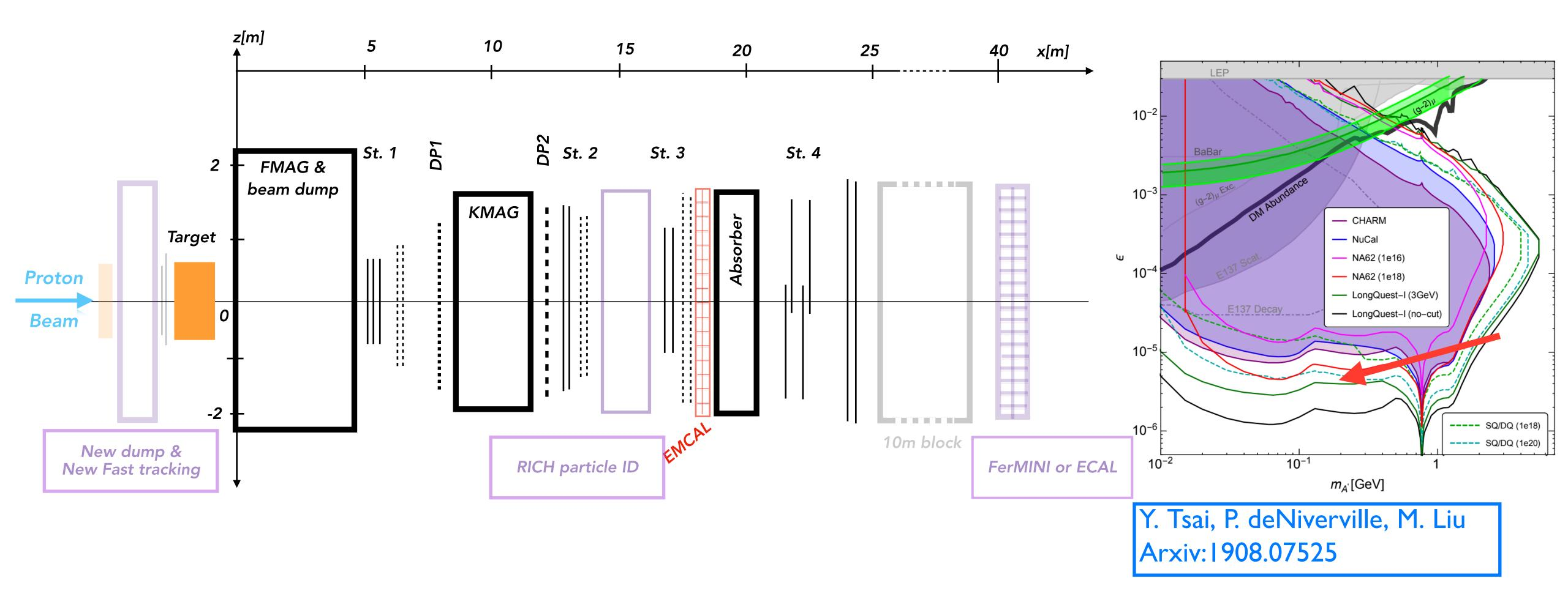
• Future upgrades of DarkQuest - LongQuest: adding particle ID detector, new dump and new fast tracking, and ECAL, to further extend the coverage and sensitivity; explore this for Snowmass
